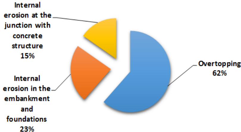
Main causes of Dam accidents and incidents in Burkina-Faso (2015's survey)
