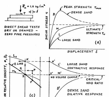
Plots of direct shear tests on dense and loose sand from the classic publication by Casagrande (1975)
