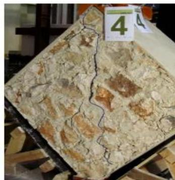
Figure 8 : Essai de compression diagonal [Milosevic, 2012]
